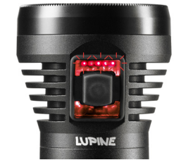
red + red blinking: battery empty
